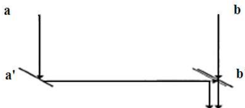
Figure 1. Diagram of an optical control system for small angular displacements
